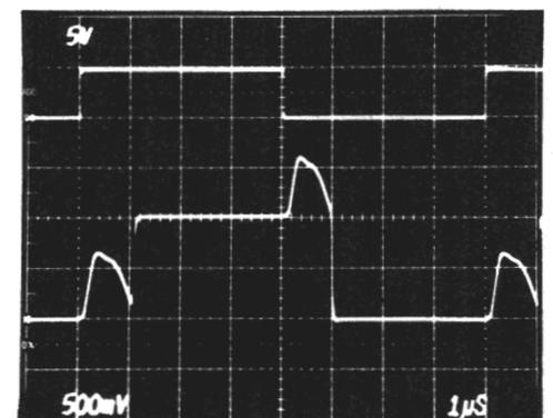
$R_L = 1M\Omega$ ,  $C_L = 10pF$ ,  $V_1 = -500mV$ ,  $V_8 = +500mV$
